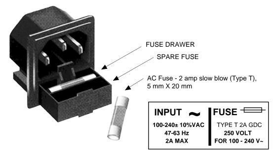
FIGURE 2.3 Fuse Location and Spare Fuse
