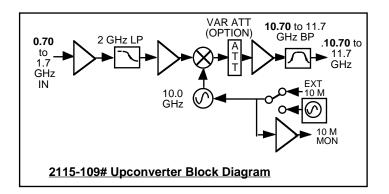
FIGURE 1.2 Model 2115-109# Upconverter Block Diagram
